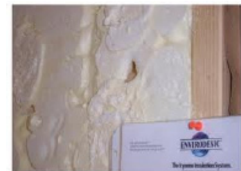
Closed cell (above) and open cell (below) foam insulation.
