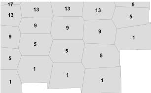
The Image effective area layer consists of adjacent polygons within a project area representing the closest image location. This layer can be used to hyper-link to non-georeferenced images. This layer can be constructed from the Photo centers layer by creating Thiessen or Voronioi polygons. This layer is optional for the standard.
