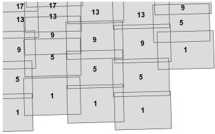
The Image extents layer consists of overlapping polygons of the extent of each photo exposure. This layer can be used for display of the actual area captured in the image. This layer is optional for the standard.
