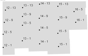
The Photo centers layer consists of point locations of the center of each photo exposure. This layer can be used to search and display photo locations as well as creation of flight index maps. This layer is required for the standard.
