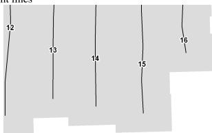
The Photo flight lines layer consists of the approximate flight lines with the vertexes at each photo center. This layer is useful in displaying the flight pattern and determining adjacent photo locations. This layer is optional for the standard.
